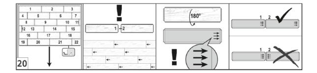
Arrows are printed on the back of each panel, which must be respected when joining the two short sides of the panel. Installation is only possible if all arrows have the same orientation. It is not possible to join two panels together on the short side with their arrows pointing in different directions.
