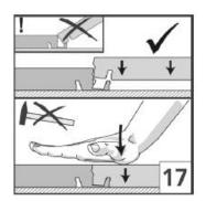
Whenever panels are assembled, the appropriate force must be applied to join them together. Do not use a hammer or tilt the panel to be joined. Do not apply any additional load to the laid surface until the adhesive has hardened. It's recommended to walk on the glued floor after a minimum of 90 minutes.
