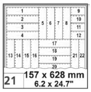
Panel (1) should be placed in the back corner of the room. Before this, the lip of the groove must be broken on one short and one long side, indicating the two boundaries of the room (walls). Between the walls and the laminate floor, a distance of approx. 12 mm must be maintained between the edges using spacers.
