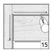
Irrespective of the installation method, each panel must be glued to all adjacent panels. To do this, a bead of glue is applied to the panels already in place. The suspended installation will not be affected
