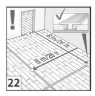
For installation surfaces with a length or width of more than 8m and in crooked rooms, expansion joints/strips (at least 2cm wide) are required. Only then can the floor expand or contract as the climate changes. Please note this is also applicable for a cross-room installation. Here, the area in the door frame must be interrupted with an expansion joint/strip. Expansion joints can be expertly covered with appropriate accessories.
