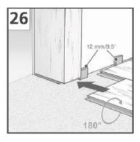
For heating pipes, holes that are 3cm larger than the pipe diameter must be recessed. Saw out, glue, fit and fix with a wedge until the glue has hardened. Then cover recesses with radiator cuffs. Shorten the wooden door frame so that a panel with impact sound insulation incl. 2 - 3mm distance below it fits. Remove spacer wedges after installation.
