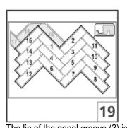
First of all, at least panels (1) to (7) must be laid in the order indicated. To do this, panel (1) is placed anywhere in the room without one lip of the groove being broken. The groove lip of panel (2) is broken on any short side. When holding the panels (1) and (2) together, make sure that the two panels can be assembled as accurately as possible. If this is the case, apply a bead of glue to a piece of the long side of panel (1) where panel (2) will rest against panel (1).
