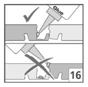
The glue bead is applied to the side of the connection on the panel that is already in place and not on the panel to be applied or on the bottom of the connection!
