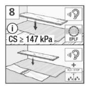
For wooden substrates no PE foil may be laid. Before laying on mineral subfloors (concrete, screed, etc.), a suitable vapor barrier film must be installed to protect against moisture. On all substrates, a suitable underlay is recommended (pressure stress min. 147 KpA, e.g.1006 Premium Sound and 1004 Silenced Board).
