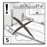
The flooring is laid floating and must not be glued, screwed, nailed or otherwise fixed to the subfloor. The placement of very heavy objects, e.g. from fitted kitchens, also has a fastening effect. Install fitted kitchens / built-in cupboards before installation. Lay the floor only up to the back of the baseboard panel.
