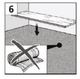
Carpets must always be removed. The carpet underneath the laminate causes a resilient movement and too much when walking on the laminate surface. The Pressure in the edge area destroys the tongue and groove connection and leads to a joint formation. The carpet must also be removed for hygienic reasons. Moisture may lead to the formation of mold and bacteria.
