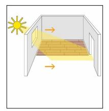
Lay the boards lengthwise to the main light source and thus towards the incoming light. The boards should be installed/laid from left to right. The boards must be floating.
