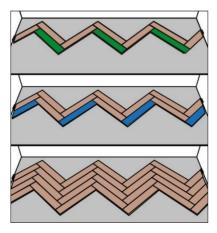
Continue from the left to the right and install all the A-panels in the second row. Now work in the opposite direction, from the right to the left and install all the B-panels in the second row. To do this, press down on the short side of the plank until it engages completely. Finish with a piece of panel cut to size. Install additional rows to complete four full rows.
