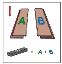
Two different types of panels are used to install the herringbone pattern. These panels are referred to as A- and B-panels. Each box contains A and B planks. To differentiate between them, the A-panels are marked on the back side.
