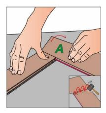
Next panel is an A-panel. Again, press the long side of the new A-panel at an angle against the short side of the previous B-panel and fold down. Continue like this as many panels as may fit along the starting wall. If necessary, also use a rubber hammer during installation to ensure that the planks are fully clicked into place. But be careful not to damage the click connection.
