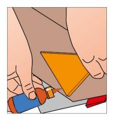
It is recommended to use glue for the click-connections to install the smallest pieces of panels.
