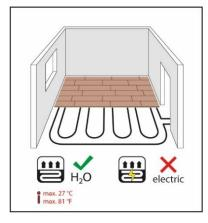
When laying on warm water underfloor heating systems, the screed must be produced in accordance with DIN18353 and heated to the required thickness (DIN EN1264 and DIN4725). The temperature on the surface of the flooring must not exceed 27 °C.
