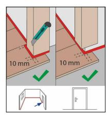
Wooden door frames can be shortened. Place a panel with the decor side down against the frame. Now shorten the door frame with a suitable saw along the panel. Then simply slide the panels under the door frame with the decor side up. In the case of door frames that cannot be shortened, cut the panel to size accordingly and observe the minimum 10 mm circumferential distance for the expansion joints.
