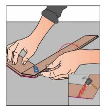
Continue with a B-panel. Press the long side of the B-panel at an angle agaist the short side of the previous installed A-panel. Fold down the B-panel flat to the floor to lock the panels tightly together. Check that the panels form a continuous line. If necessary, use a rubber hammer during installation to ensure that the planks are fully clicked into place. But be careful not to damage the click connection.
