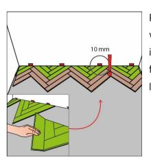
Put the adjusted rows (in the picture green marked) into place. If you use version 1, connect the cut starting panels to form triangular shapes. Start installing the triangles from the left corner. It is recommended to use glue to fix the smallest parts (click-connections) of the triangles. Make sure that you leave a gap of 10 mm to the wall.
