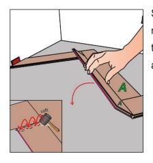
Start the next row with an A-panel. Place the new panel against the previous row and fold down. To do this, press down on the short side of the plank so that the click connection engages completely. If necessary, tap lightly with a rubber hammer.
