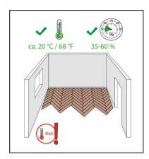
Please note that typical living room temperatures must prevail throughout the year (VOB, Part C, DIN 18365, DIN EN1264, DIN 4725). The room air temperature should be approx. 20 °C, the relative humidity should be between 35-60 %.
