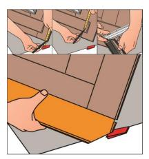
For the last row you need the planks from the first four rows (orange marked in the picture). Optionally you have to measure and cut the panels.
