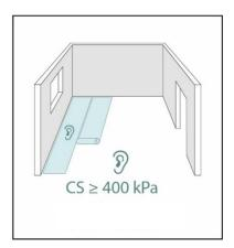
The use of a suitable impact sound insulation for vinyl floors is necessary. Please use an impact sound insulation with a pressure load of min. 400 kPa.
