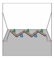
Check the first row of panels is centered along the starting wall. Make sure that the distance to the walls on both sides are less than the length of one panel. If not, add a panel at the right side.
